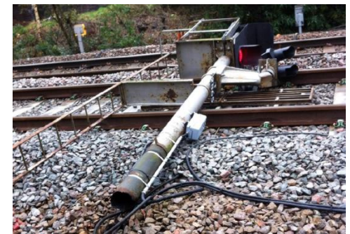
Collapsed signal post at Newbury. Source: RAIB, 2015.
