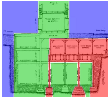
Section of the first, ground, and basement levels of One Times Square showing the physical interfaces forming the Subway UUMI and the building, with presumed property interfaces overlaid. Source: Based on information within Purdy, 1909.
