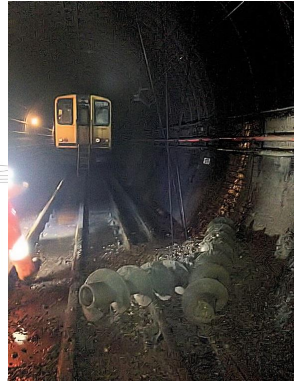
Auger sections and debris on the track. Source: RAIB, 2014.
